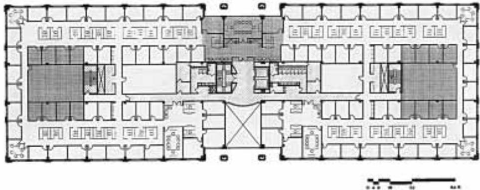
**Figure 90.** Ground floor mechanical plan of the DMS office building; illustrative of the complexity of HVAC systems in this scale of building.
